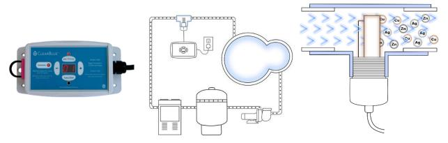
ClearBlue adds microscopic mineral ions to the water consisting of silver, copper and zinc. It does this by conducting a weak electrical charge inside the mineral cell across a set of electrodes that are added to the plumbing with a tee. As the electrical charge conducts through the water from one electrode to the other, the ions are released into the water.
